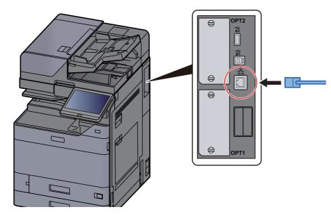
2 Connect the other end of the cable to the hub or the PC.
